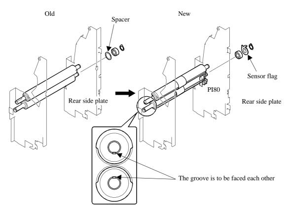
Direction of the upper/lower part of the folding roller in attachment.
